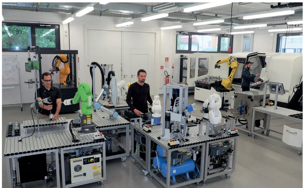
TU Graz smart factory is equipped with state-of-the-art machining, additive manufacturing centers and industrial robots from various manufacturers arranged in mobile, self-sufficient workstations.
